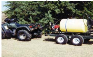
ATV Towable Tank Sprayers
